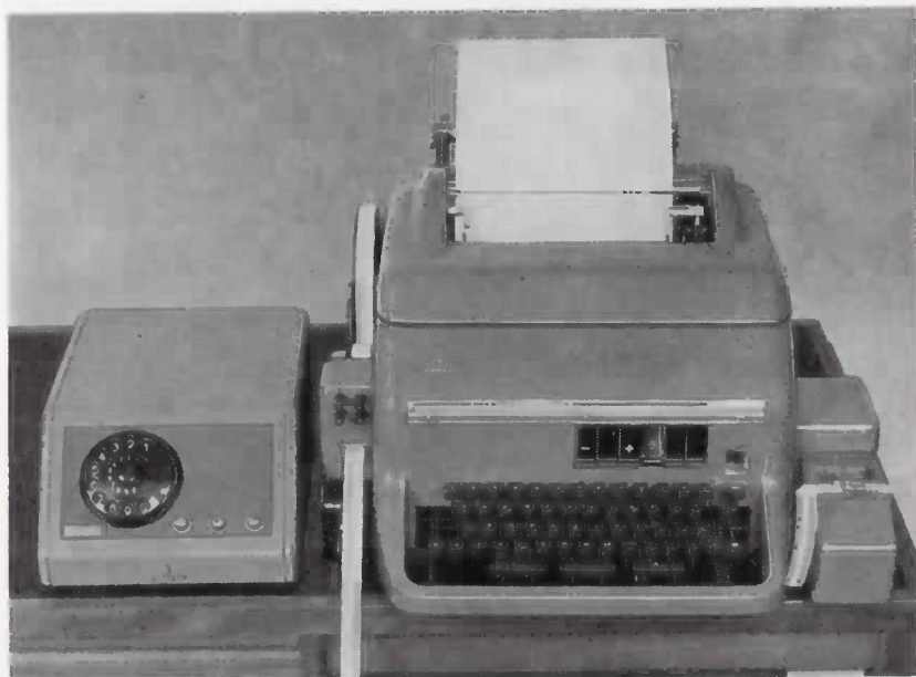
Fjernskriveinstallation. Maskintype T 100
