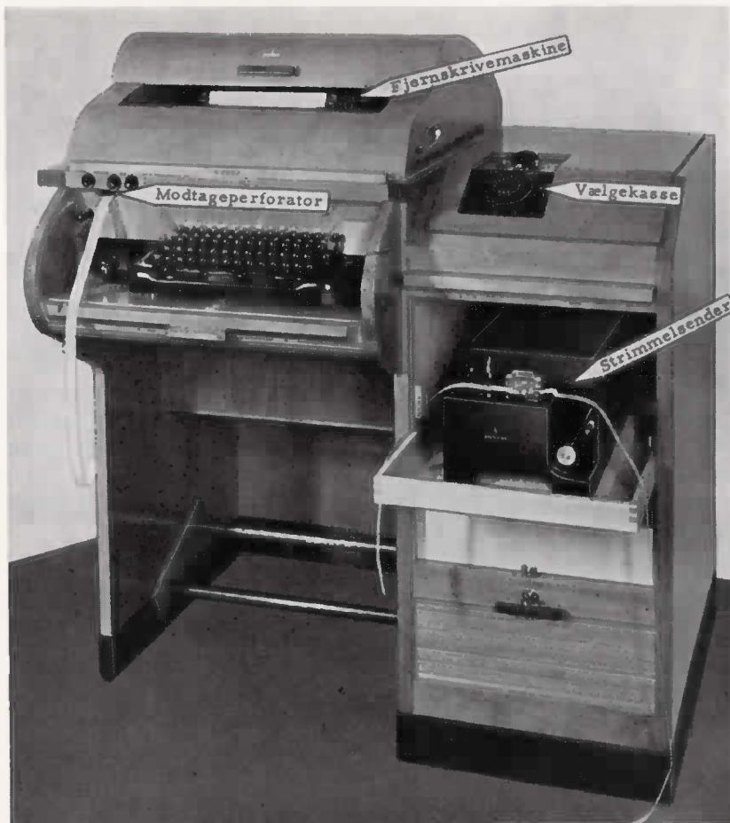
Fjernskriveinstallation. Maskintype T 37
