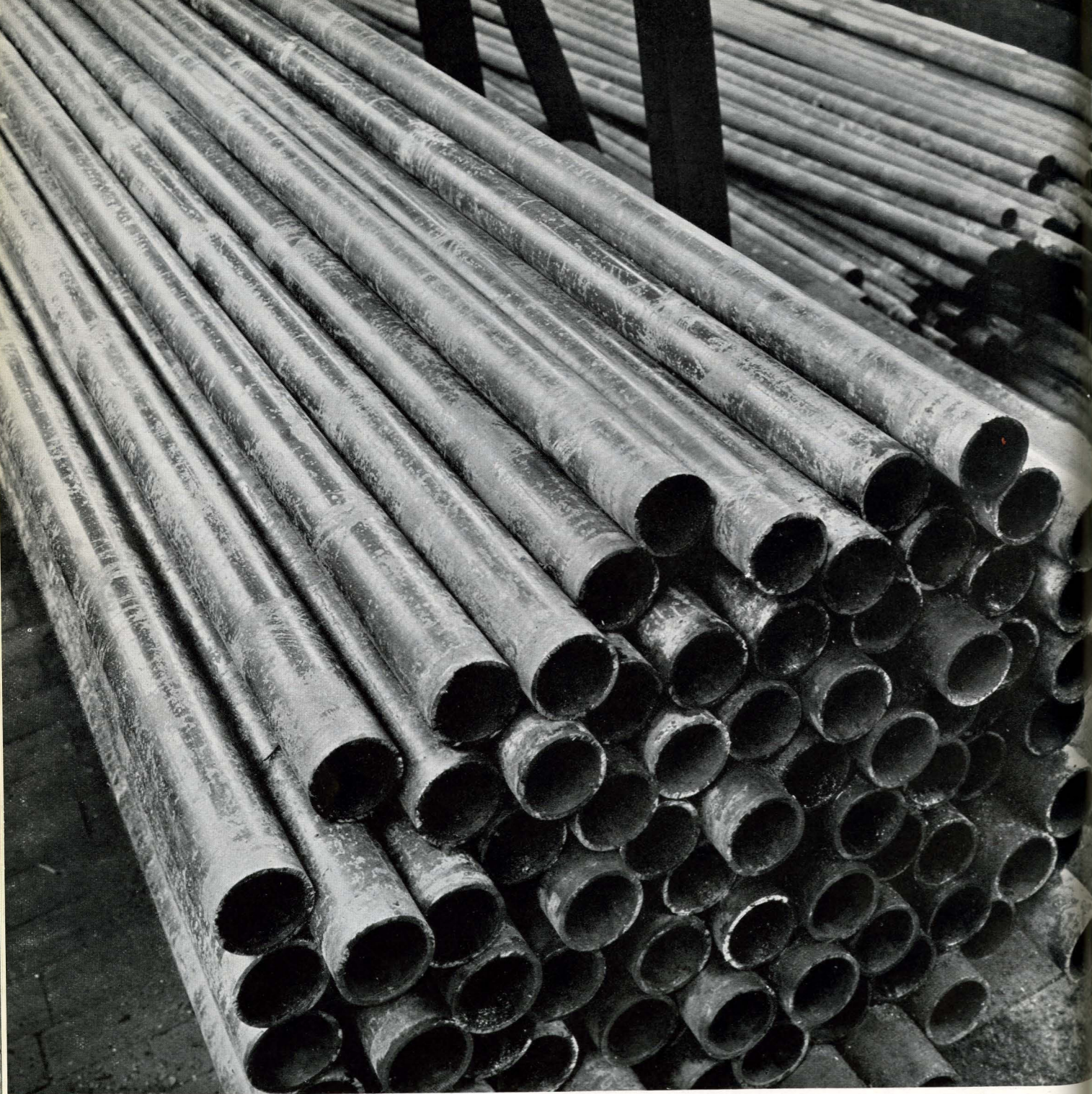
Descaled tubes after 12 months' service from Locomotives running on partially softened water. Note absence of corrosion and the presence of 'mill' scale. London & North Eastern Railway Co., Ltd.
