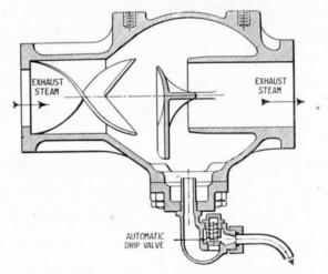
Fig. 59.—Section through Grease Separator and Drip Valve.
