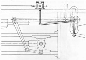
Fig. 216 — Mechanical Lubricator driven from Expansion Link of Walschaerts Valve Gear. (See also Fig. 231.)
