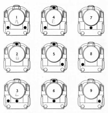
Fig. 11.—Head-Lamp Code for Classifying Trains.
