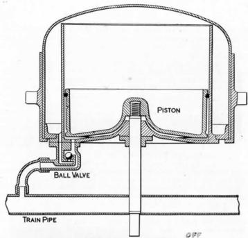
FIG. 181.—AUTOMATIC VACUUM BRAKE, "ON."
