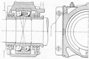
Fig. 73.—S.K.F. Roller-Bearing Axlebox for Inside Journals.
