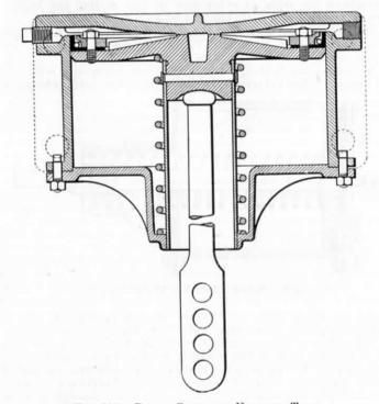
Fig. 207.—Brake Cylinder, Vertical Type.
