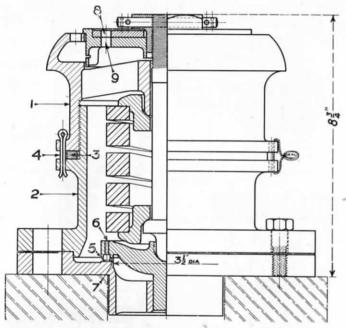
Fig. 44.—Ross "Pop" Safety Valve for Locomotive Boilers.
