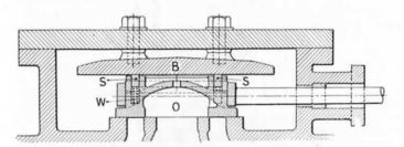
Fig. 101.—Richardson Balanced Slide Valve for Locomotives.
