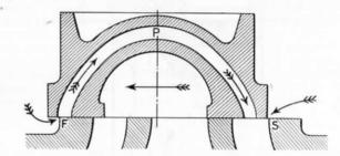
Fig. 100.—Locomotive Slide Valve (Allan or Trick Pattern).
