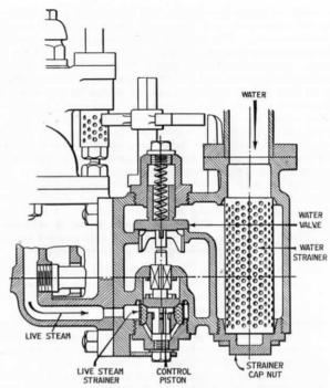
FIG 58.—Section through Water Inlet Valve and Operating Piston and Water Sieve.
