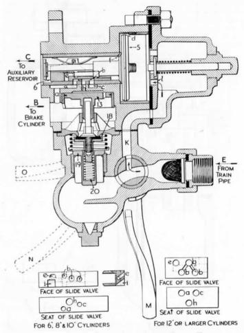
Fig. 205.—Westinghouse Quick-Acting Triple Valve.
