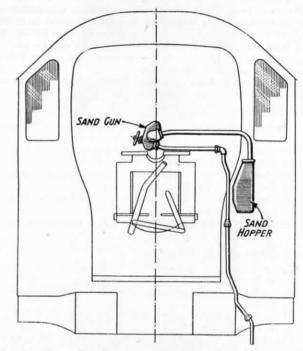
Fig. 24.—Sand Gun Fittings used on L.M.S.R. Locomotives.
