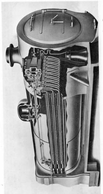
STEAM "MELESCO" SUPERHEATING APPARATUS AND TANGENTIAL SHOWING LOCOMOTIVE BOILER
