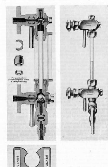
Fig. 46.—Details of Dewrance Water-Gauge Fittings for Locomotives.
