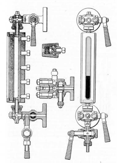
Fig. 48.—Details of Klinger Reflex Water-Gauge FITTINGS.
