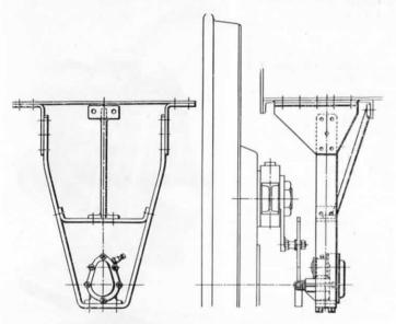
Fig. 248.—Typical Gearbox Suspension Bracket, Stone-Deuta Speed Indicator.
