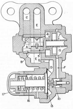
Fig. 203.—Regulating Feed Valve of Westinghouse Brake System.
