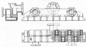
FIG. 161.—Type "A.X." Superheater Header.
