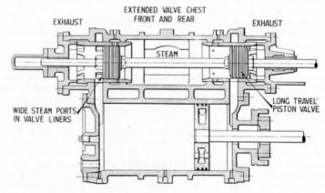
Fig. 99.—Above: Old Pattern Cylinder and Valve. Below: Cylinder Valve and Piston of New Standard Locomotives, L.M.S.R.
