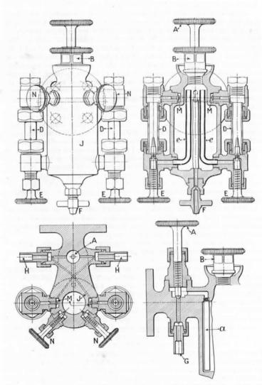
Fig. 221.—Wakefield Double Sight-Feed Lubricator with Auxiliary Feed.
