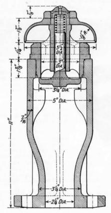
Fig. 173.—Superheater Header Relief Valve, Southern Railway.
