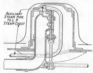
Fig. 155.—Regulator and Auxiliary Steam Pipe, Compound Locomotive, L.M.S.R.
