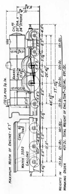
Fig. 291.—"C1" Class 4.4-2 Locomotive, L.N.E.R.
