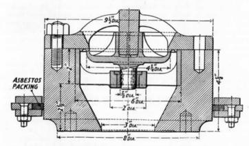
FIG. 163.—Anti-Vacuum Valve, L.N.E.R.
