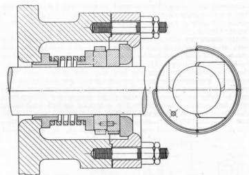
Fig. 122.—Packing with Cast-iron Rings, (United States Metallic Packing Co. Ltd.)
