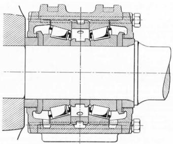
Fig. 70.—Timken Axlebox for Inside Journals, as used on Locomotive Leading Bogies, containing Two Single-Row Timken Tapered Roller Bearings
