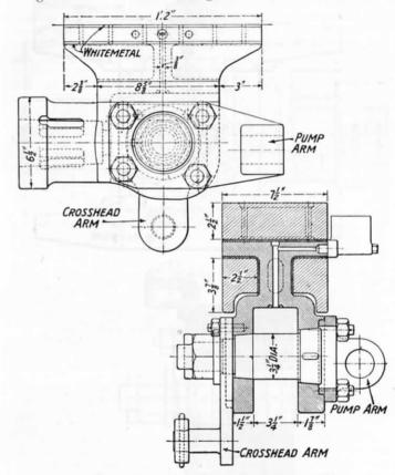
Fig. 124.—Three Slide-Bar Crosshead, Southern Railway.
