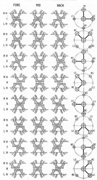
Fig. 258.—Relative Positions of Cranks, Valves, and Slide Rods.
