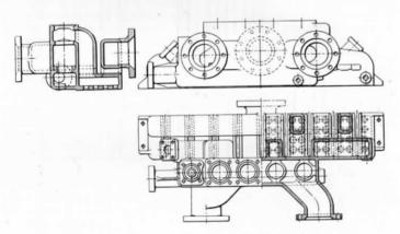
Fig. 162.—The "MeLeSco" Multiple Valve Regulator.
