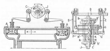
Fig. 108.—Section through EXHAUST VALVES.
