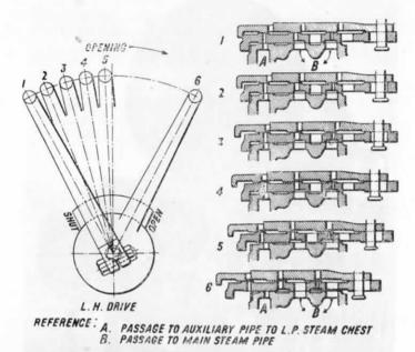
FIG. 157.—DIAGRAM SHOWING METHOD OF ADMITTING LIVE STRAM TO L.P. CYLINDERS, COMPOUND LOCOMOTIVE, L.M.S.R.
