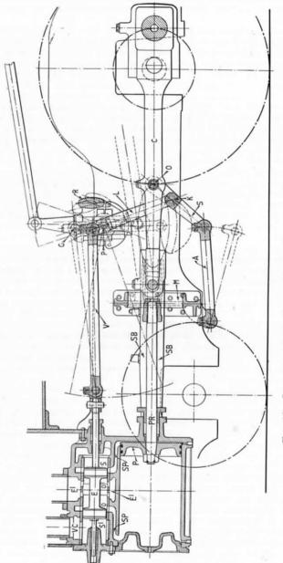
92.—Layout of Joy's Radial Valve Motion for Locomotive
