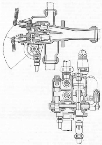
Fig. 193.—Top: Section through Nozzles, Steam, Exhaust, AND TRAIN PIPES. Bottom: SECTION THROUGH STEAM AND AIR ADMISSION VALVES.
