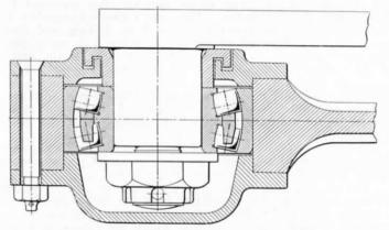
Fig. 77.—Roller-Bearing Return Crank.
