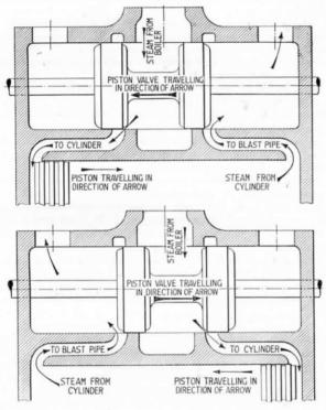
Fig. 260.—Relative Positions of Steaming and Exhausting Edges; Inside Admission Piston Valves and Ports.
