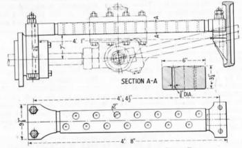
Fig. 126.—Crosshead for Single Slide Bar.
