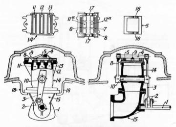
Fig. 41.—Details of L.M.S.R. Regulator Valve and Fittings in Dome.
