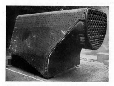
Fig. 36.—Combustion Chamber Firebox, 4-6-2 Type Engine, L,M,S,R,
