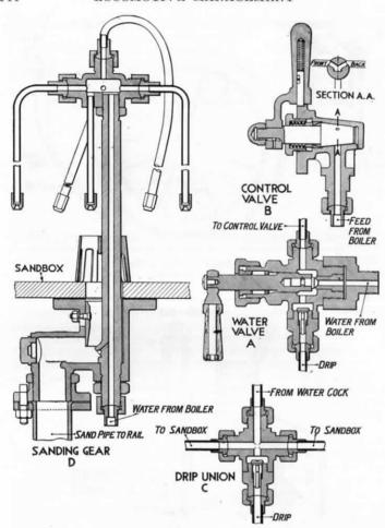
FIG. SO.—DETAILS OF LAMBERT WET SANDING GEAR.
