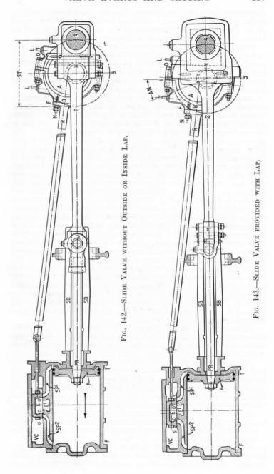
the exhaust has closed to the time that the valve opens to steam at the point of admission. All these events occur at both ends of the cylinder during the course of one revolution, and will be
