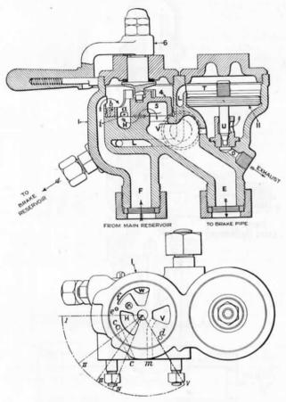
Fig. 202.—Sectional and Plan Views of Driver's Brake Valve.
