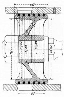
Fig. 102.—Latest Type of PISTON VALVE, L.M.S.R.
