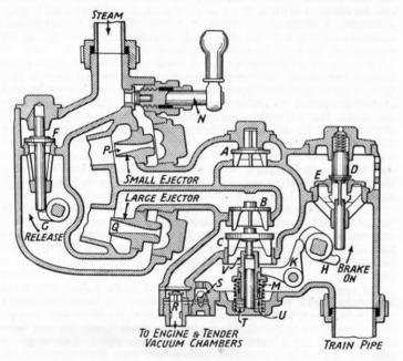
Fig. 192.—Diagrammatic View of "S.J." Ejector.
