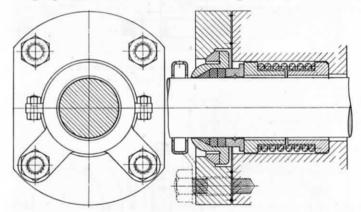
FIG. 121.—United States Metallic Packing (Air-Cooled Type).
