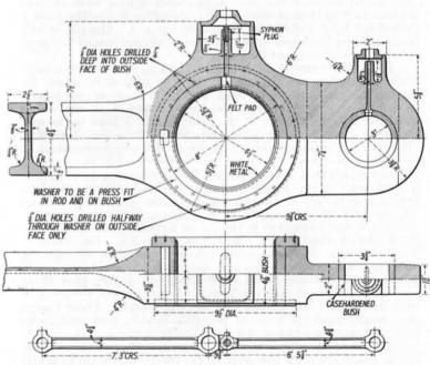
Fig. 84.—Details of Coupling Rods of 4-6-2 Type Express Engine, L.M.S.R.
