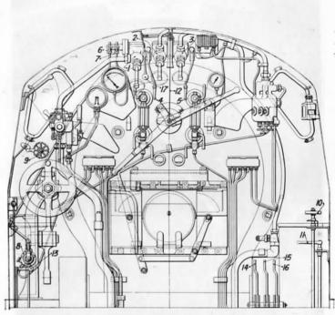
Fig. 279.—Arrangement of Footplate Fittings: Southern Railway "Schools" Class Locomotive.
