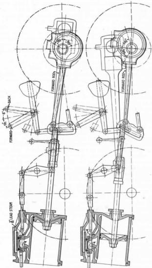
Figs. 253 and 254.—Diagrams showing Relative Crane, Piston, and Valve Positions in Forward Gear (Back and Top Dead Centres).
