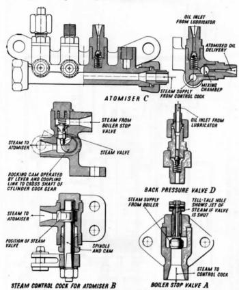
Fig. 237.—Atomiser Cylinder Lubrication System fitted to L.M.S.R. Engines.
