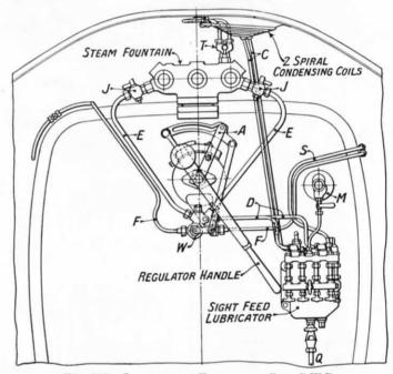
Fig. 232.—Lubricating Fittings in Cab, G.W.R.
