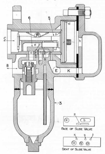
Fig. 206.—Westinghouse Improved Triple Valve.
