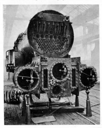
Fig. 156.—View of Front End, L.M.S.R. Three-Cylinder Compound Locomotive, showing H.P. and L.P. Cylinders and Steamchests.
