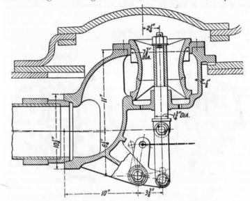
FIG. 40.—L.N.E.R. BALANCED REGULATOR VALVE.
