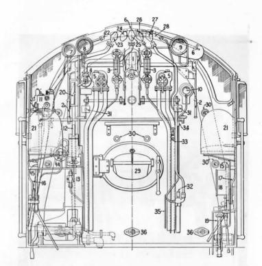
Fig. 277.—Arrangement of Footplate Fittings: L.N.E.R. "A 4" CLASS LOCOMOTIVE.
