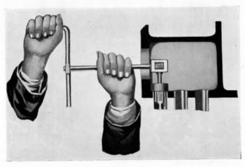
Fig. 167.—Method of Expanding Superheater Tubes.
