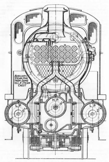
Fig. 154.—Cross-Section through Cylinders and Smokebox, Three-Cylinder Compound Locomotive, L.M.S.R.
