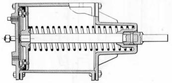
Fig. 208.—Brake Cylinder, Horizontal Type.
