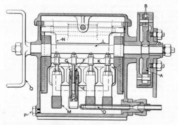
Fig 229.—Silvertown Mechanical Lubricator in Sectional Elevation.
