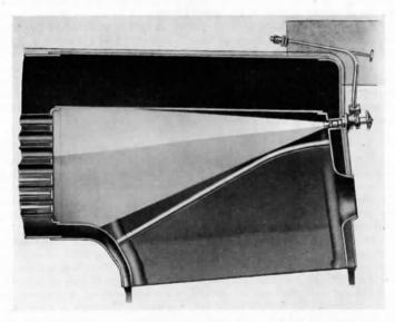
Fig. 23.—Sectional View of a Firebox fitted with Clyde SOOT BLOWER ON THE BACK PLATE.
