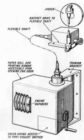
Fig. 15.—Apparatus for Recording Engine Number and Amount of Coal Delivered to Tender.
