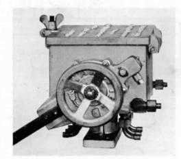
Fig. 215.—Wakefield No. 7 Pattern Mechanical Lubricator.
