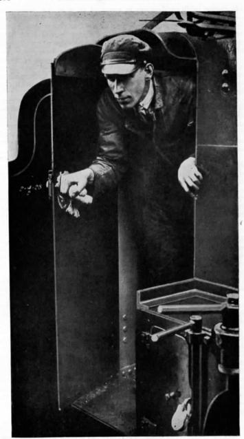
FIG. 179.—CORRIDOR TENDER, L.N.E.R. INTRODUCED TO ALLOW OF CHANGING ENGINEMEN DURING NON-STOP RUN, LONDON TO EDINBURGH.
