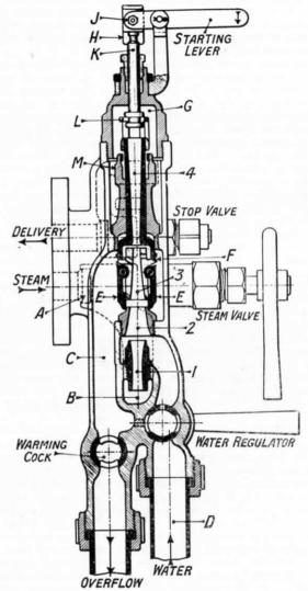
Fig. 52.—Gresham Patent Hot-Water Combination Injector,
