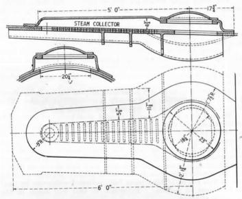
Fig. 42.—Sectional Elevation, Plan and Cross-Section of Steam-Collecting Device, L.N.E.R.
