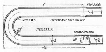
Fig. 172.—Electrically Butt-Welded Return Bend of "Swindon" Superheater.
