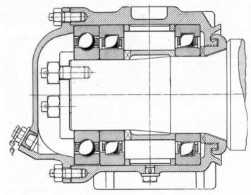
Fig. 75.—Hoffmann Roller-Bearing Axlebox for Outside Journals, with Bronze Pads for End Location,
