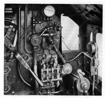
Fig. 250.—G.W.R. Speedometer, Cab Fittings.
