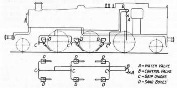
Fig. 81.—Arrangement of Lambert Wet Sanding Gear on Locomotive.
