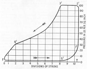
Fig. 149.—Diagram taken from Engine at Low Speed.
