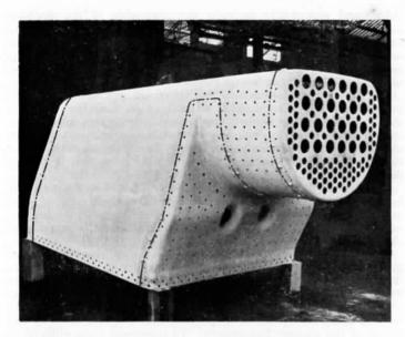
Fig. 35.—Welded Firebox with Combustion Chamber (Vulcan Foundry).
