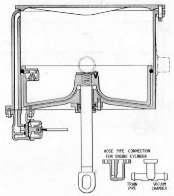
Fig. 185.—"E" Type Cylinder (Separate Pattern).
