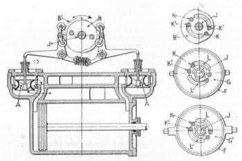
Fig. 107.—Section through Cylinder AND INLET VALVES.
