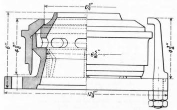
Fig. 45.—Automatic "Jumper" Blast-Pipe Top, G.W.R.
