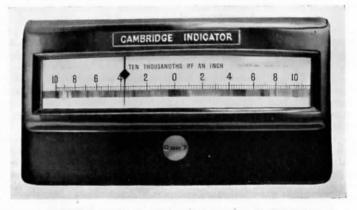
Fig. 175.—Indicator of Cambridge Thermo-Electric Pyrometer for Superheated Locomotives.
