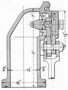
Fig. 37.—Double-Ported, Flat Type Regulator Valve.
