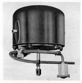
Fig. 189.—External View of Westinghouse Quick-Service Valve.
