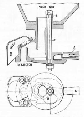
Fig. 79.—Section and Plan of Sandbox AND ATTACHMENTS.
