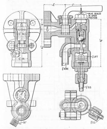
Fig. 43.—Automatic Continuous Blowdown Valve.
