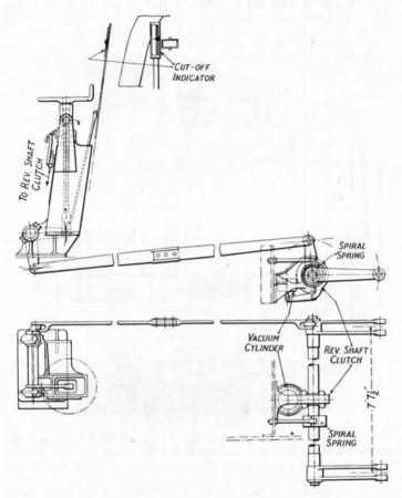
Fig. 95.—Screw Reversing Gear of L.N.E.R. 4-6-2 Express Locomotive.
