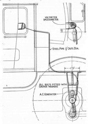
Fig. 252.—Arrangement of Driving Mechanism and Generator; Armoured A.C. Cable and Speedometer in Cab, G.W.R.
