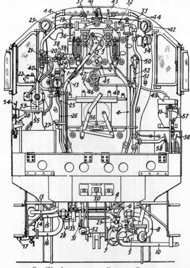
Fig. 275.—Arrangement of Footplate Fittings: L.M.S.R. "5 X" CLASS LOCOMOTIVE.
