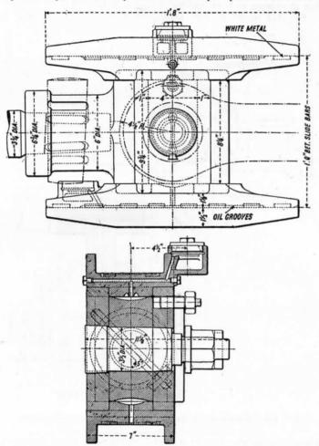
Fig. 125.—Crosshead for Outside Cylinders with Two Slide Bars.
