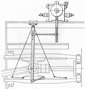
Fig. 217.—Mechanical Lubricator driven from Crosshead.
