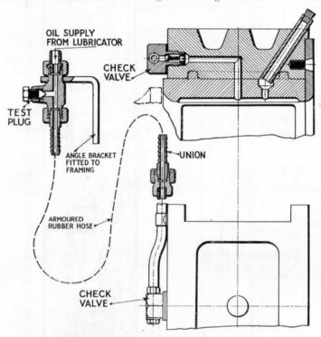
Fig. 219.—Method of Applying Forced Feed Lubrication to Locomotive Axleboxes with Overhung Springs.
