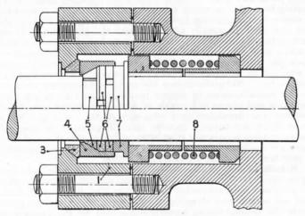
Fig. 118.—Spring-Controlled Metallic Packing.
