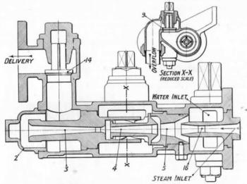
Fig. 51.—Gresham Under-Footplate Type Injector.
