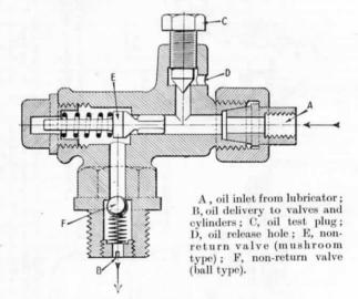
Fig. 227.—Combined Check and Test Valve for Wakefield Mechanical Lubricators.
