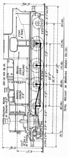
Fig. 288.—" 7200" Class 2-8-2 Tank Engine, G.W.R.
