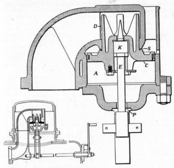
Fig. 39.—Details of the "Servo" Regulator VALVE FOR LOCOMOTIVES.
