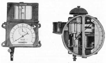
FIG. 242.—THE TELOC AND HASLER SPEED INDICATORS AND Recorders for Locomotives (Hasler Telegraph Works)
