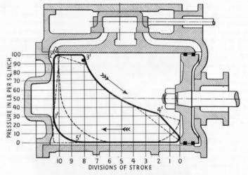
Fig. 150.—Indicator Diagram Superimposed on Locomotive Cylinder showing Action of Steam.
