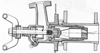
Fig. 20.—Details of Diamond Soot Blower for Locomotive Boilers.
