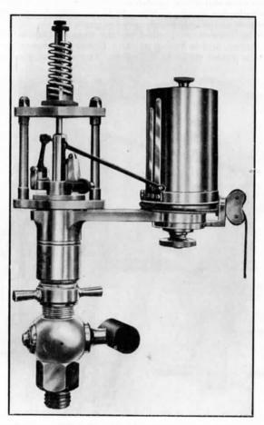
Fig. 148.—Crosby "New No. 2" Type Indicator with Outside Spring.
