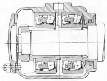
Fig. 72.—S.K.F. Roller-Bearing Axlebox for Outside Journals.
