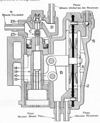
Fig. 209.—Westinghouse Straight Air Brake Application Valve (Proportional Valve).
