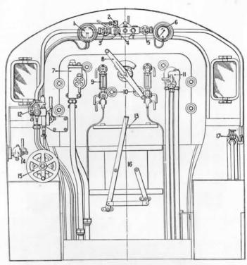
Fig. 283.—Arrangement of Footplate Fittings: 4-4-0 Type Locomotive, Coras Iompair Eireann.
