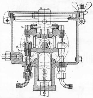
Fig. 225.—Wakefield Mechanical Lubricator (Single-Acting Pattern).
