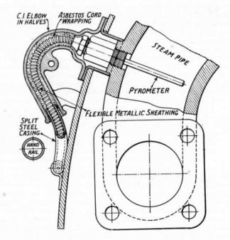
Fig. 176.—Arrangement of Thermo-Couple for Cambridge Pyrometer,
