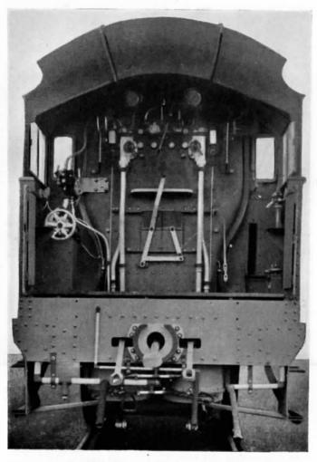
Fig. 282.—View of Footplate Fittings: 4-4-0 Type Locomotive, Coras Iompair Eireann.
