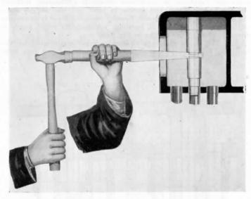
Fig. 168.—Method of Extracting Superheater Tubes.
