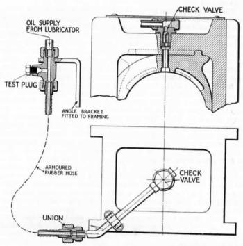
Fig. 218.—Method of Applying Forced Feed Lubrication to Locomotive Axleboxes with Underhung Springs.
