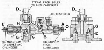
Fig. 226.—Anti-Carboniser (Wakefield Pattern).
