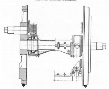
FIG. 71.—TIMKEN "CANNON" TYPE AXLEBOX FOR LOCOMOTIVE DRIVING AXLES. SINGLE TAPERED ROLLER BEARING MOUNTED ON EACH JOURNAL, HOUSED IN TUBULAR-TYPE AXLEBOX, EMBRACING THE ENTIRE AXLE BETWEEN WHEEL HUBS.
