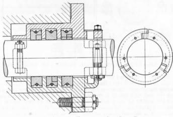
Fig. 123.—Another Type with Cast-Iron Rings, (United States Metallic Packing Co. Ltd.)
