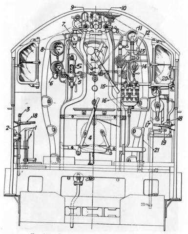
Fig. 273.—Arrangement of Footplate Fittings: G.W.R. "KING" CLASS LOCOMOTIVE.
