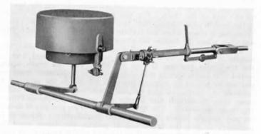
Fig. 210.—"Weslak" Slack Adjuster shown after resetting.
