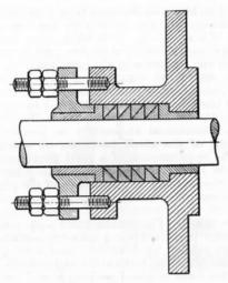
FIG. 117.—METALLIC PACKING FOR PISTON RODS.
