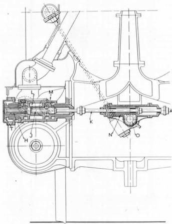
Fig. 105.—Section through Transverse Camshaft and Cams; "A.L.E." Rotary Cam Popper Valve Gear.
