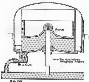
Fig. 182.—Automatic Vacuum Brake, "Off."
