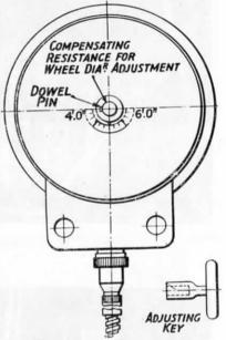
Fig. 249.—Method of Adjusting Tyre Wear, Stone-Deuta Electrical Speed Indicator.
