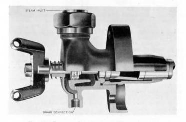
FIG. 19.—DIAMOND SOOT BLOWER: VALVE CLOSED.
