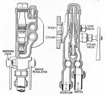
Fig. 50.—Gresham & Craven Automatic Restarting Injector.
