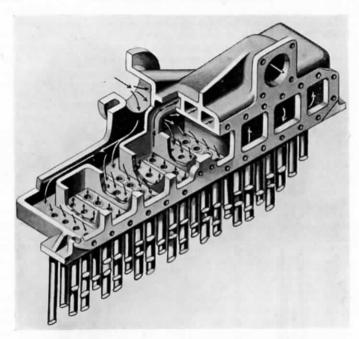
FIG. 166.—ELEMENTS EXPANDED DIRECT INTO HEADER. (Arrows indicate course of steam.)
