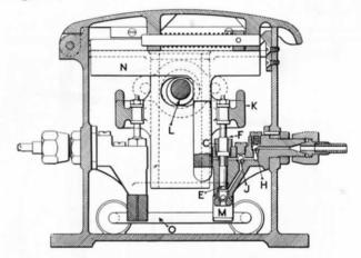
Fig. 230.—Silvertown Mechanical Lubricator in Cross-Section.
