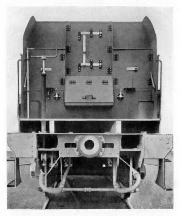
Fig. 284.—View of Tender Fittings: 4-4-0 Type Locomotive, Coras Iompair Eireann.
