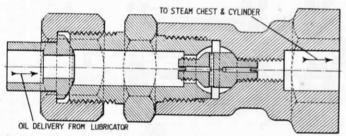
Fig. 223.—Steamchest and Cylinder Connection.
