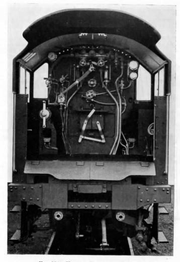
Fig. 274.—View of Footplate Fittings: L.M.S.R. "5 X" CLASS LOCOMOTIVE.
