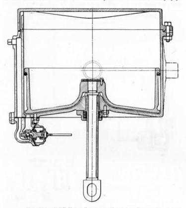
Fig. 184.—"C" Type Cylinder (Separate Pattern).
