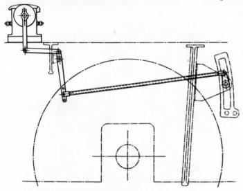
Fig. 231.—Method of Operating Mechanical Lubricator from Die Block of Walschaerts Valve Gear. (See also Figs. 216 and 217.)
