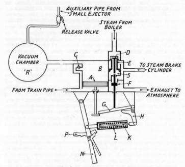
Fig. 197.—Diagram of Graduable and Automatic Steam Brake Valve Mechanism.
