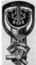
Fig. 38.—The "Joco" Com-BINED REGULATOR AND DRIFTING VALVE.
