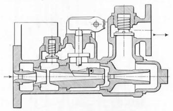
Fig. 53.—Metcalfe Hot-Water Injector, Section through Nozzles and Valves.
